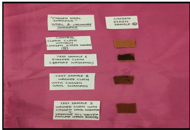
Fig. 3: Washing results of stained woolen fabric pieces having chosen stain sample B of hair colour dye crème (Loreal Paris Casting Crème Gloss Black) with chosen woolen shampoo named, Wool & Cashmere Shampoo and prepared bio-active jasmine oil driven BSANPs [13]
