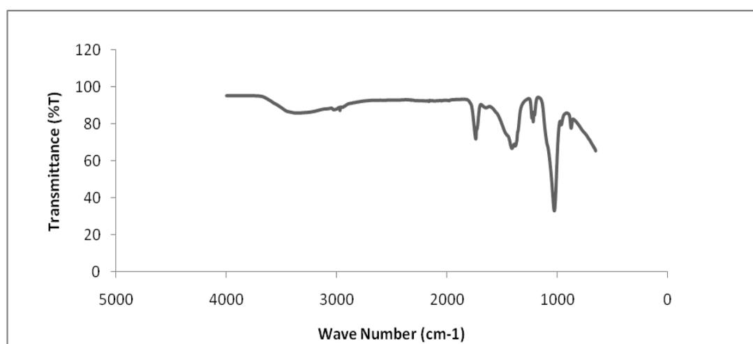
**Fig. 2:** FTIR spectrum of the Ti samples after NaOH-heat treatment soaked in modified SBF for 20 days
