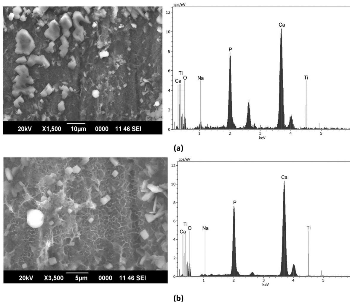
**Fig. 4:** SEM and EDX analysis of the surfaces of Ti after NaOH, heat treatments and immersion in SBF modified with (a) calcium gluconate and (b) calcium nitrate for 20 days
