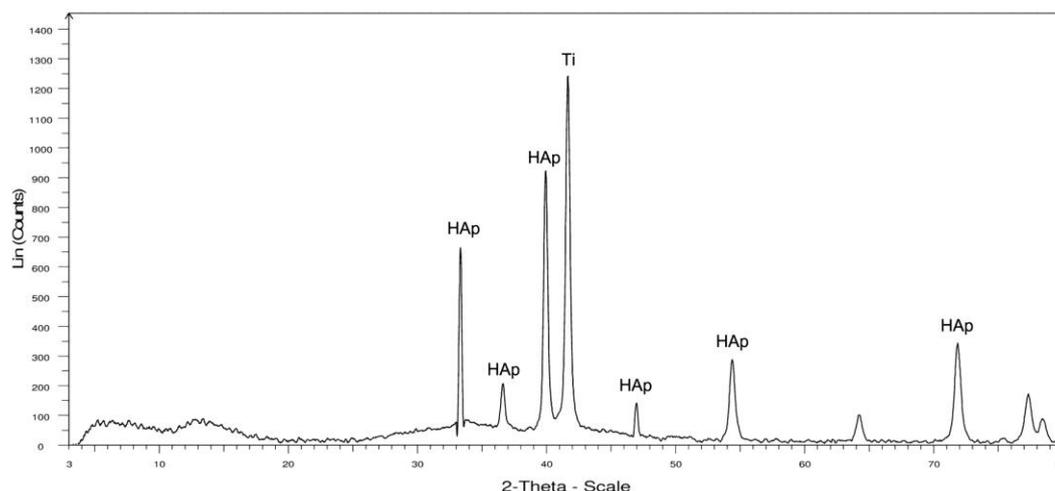
**Fig. 3:** XRD patterns of the surfaces of Ti after NaOH-heat treatments and soaked in SBF modified with calcium gluconate 20 days
