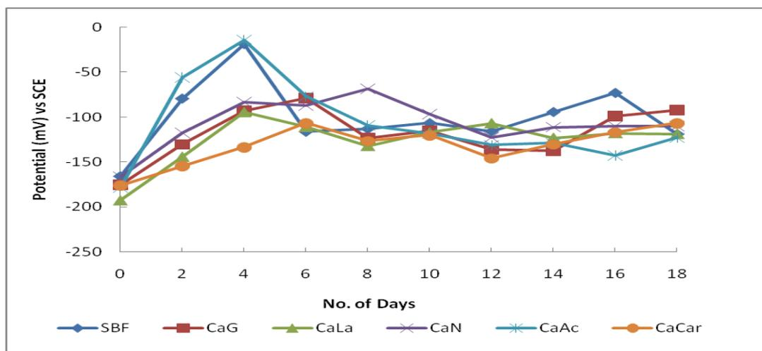
**Fig. 1:** Surface potential change for the Ti samples after NaOH-heat treatment and soaked in modified SBF for 20 days
