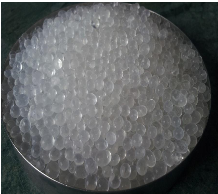
Fig. 3: Silica Gel beads [8]
