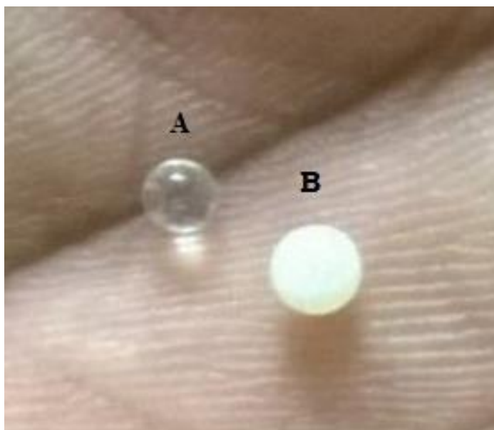
Fig. 5: Silica gel beads A: Normal silica gel bead (Transparent) B: Microbial growth in bead (white)
