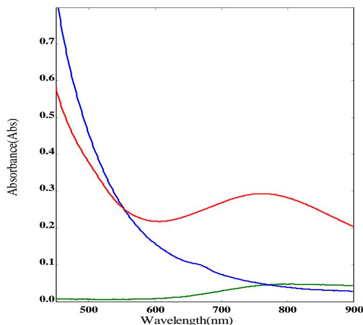
**Fig. 1:** UV-Vis spectra of synthesized CuNPs using aqueous leaf extract of *A. heterophyllum*
