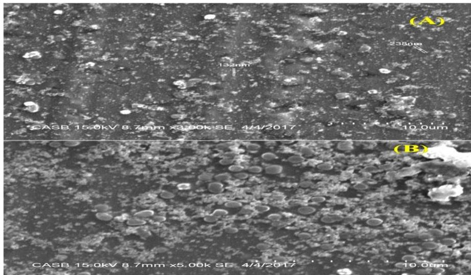
**Fig. 4:** Scanning electron micrographs of CuNPs synthesized with *A. heterophyllus* leaf extract and magnified **(A)** 8.7mm×3.00 and **(B)** 8.7mm×5.00 inset bar represents 10 µm
