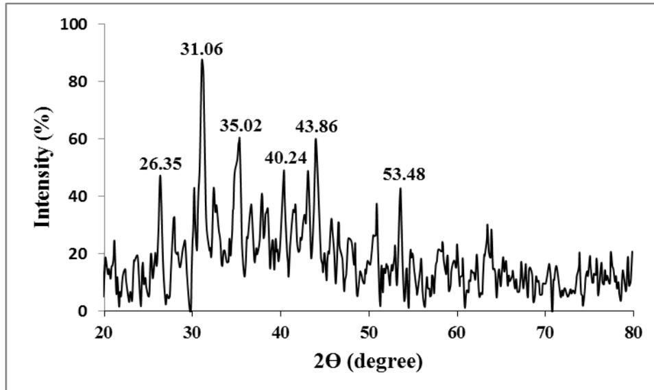
**Fig. 2:** XRD analysis of synthesized CuNPs using aqueous leaf extract of *A. heterophyllus*
