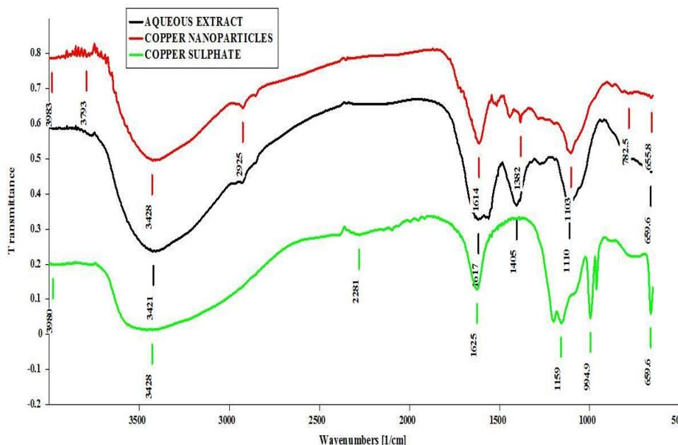
**Fig. 3:** FTIR spectrum of color variations (Black indicating Aqueous extract, Green indicating CuSO<sub>4</sub> and Red indicating Synthesized CuNPs)
