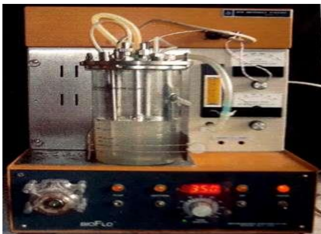
Fig. 2: Fermenter used for biotransformation
